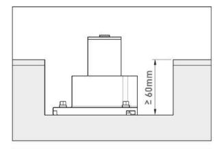
There are 3 fixing positions and 3 levelling bolts.
